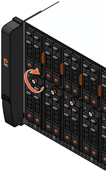
Figure 2.30 Securing the Ejector Handle
