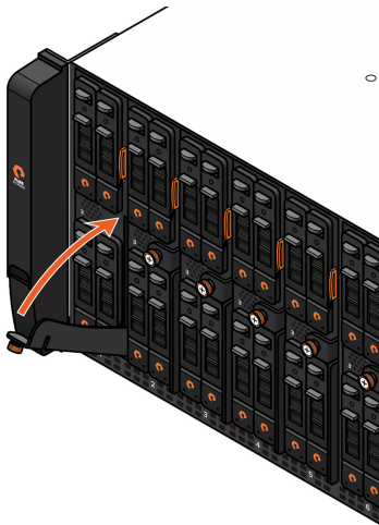
Figure 2.29 Closing the Ejector Handle
