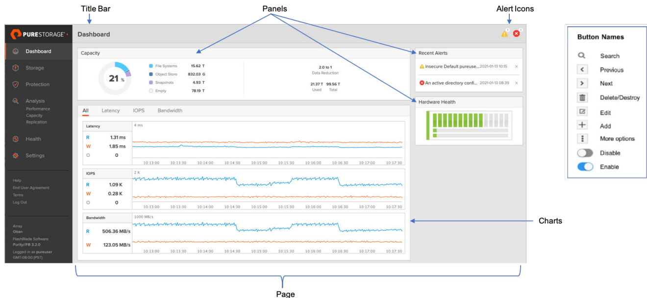
Figure 3.3 Purity//FB GUI - Page and Buttons
