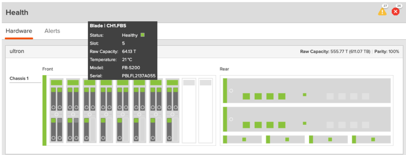
Figure 10.6 Health - FlashBlade//S Hardware Panel (Front and Rear Views)
