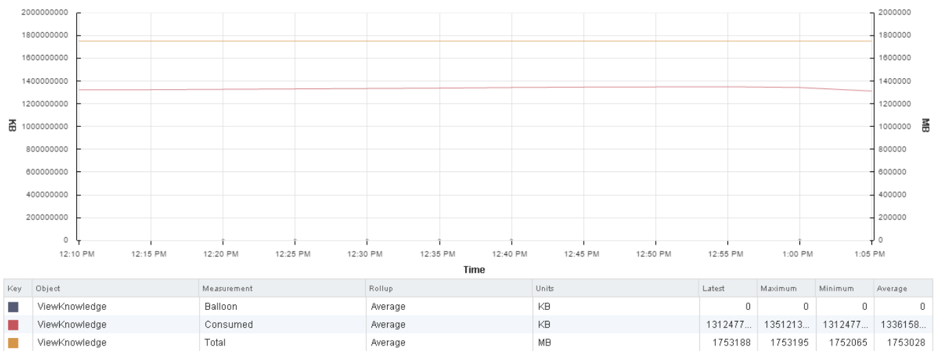
Figure 42: 7 host ESXi cluster memory utilization for 300 Knowledge Workers and 300 Power Workers during 1500 user mixed workload test. No swapping or ballooning was detected
