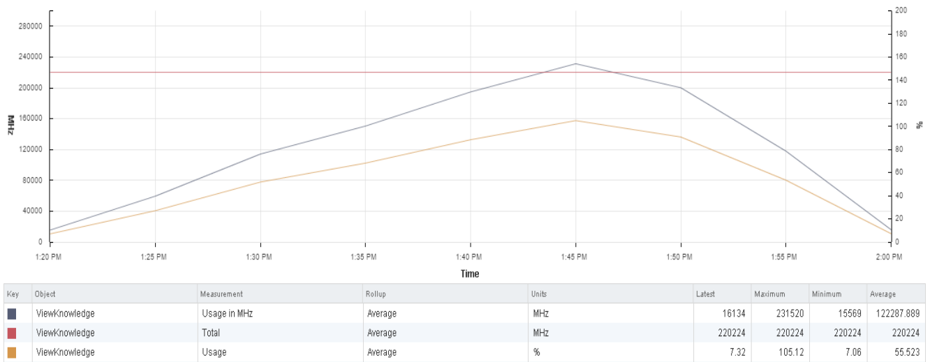
Figure 24: 4 ESXi cluster CPU utilization during 370 mixed workload Login VSI simulation
