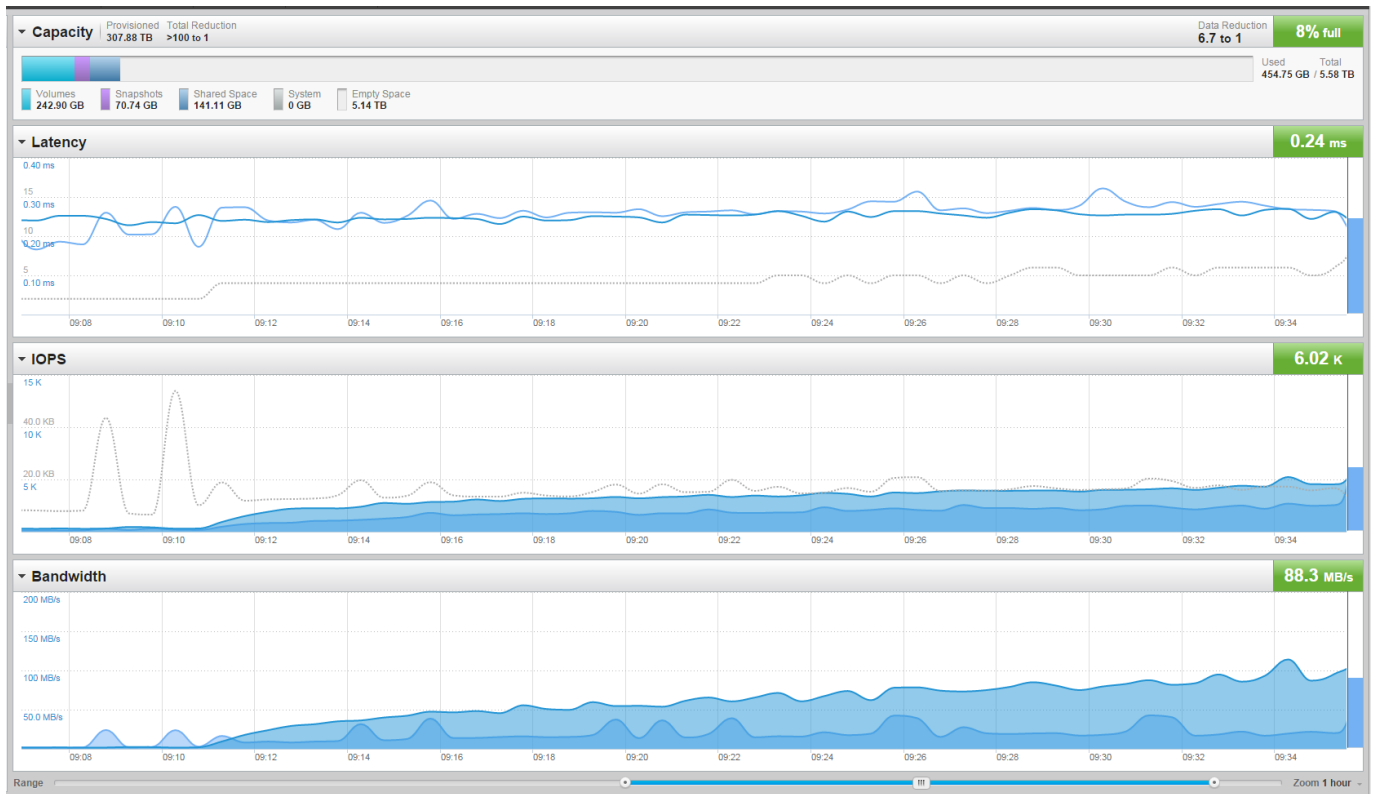
Figure 29: Pure Storage dashboard showing 370 mixed workload simulation storage performance leading up to bootstorm
