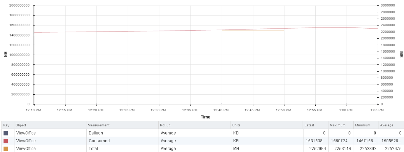
Figure 44: 9 host ESXi cluster memory utilization for 900 Office Workers during 1500 user mixed workload test
