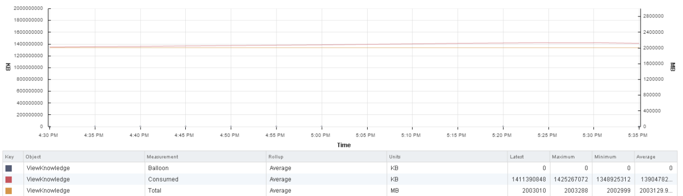
Figure 34: 8 host ESXi cluster showing memory utilization for 750 mixed workload simulation. No swapping or ballooning is noted
